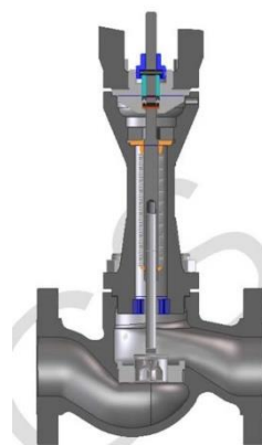
Figure 14 Schematic Diagram of MK-GS Bellows Type Valve Cover Structure
