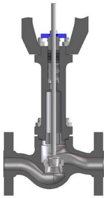
Figure 13 Diagram of the MK-GS Extended Valve Cover Structure
